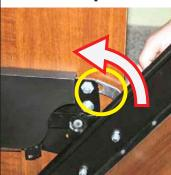
Ease the panel up and rotate the silver bracket over the top nut on the mechanism to prevent the door from closing.
