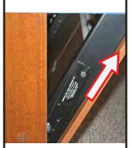
Carefully tilt and slide the front panel upwards respecting the locked angle.
